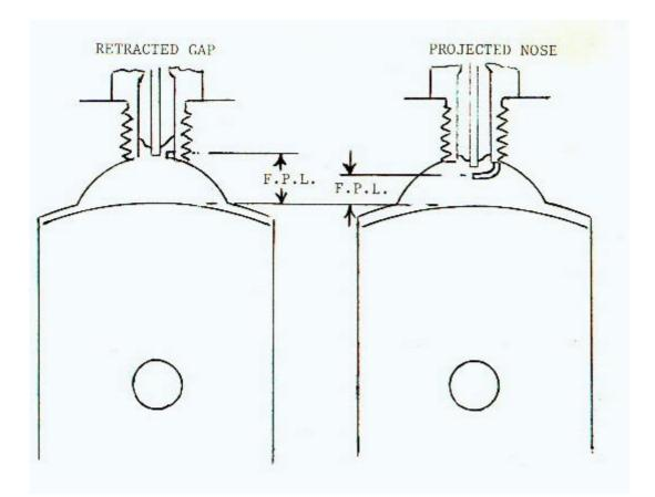
When changing from retracted gap to projected nose configuration (or vice versa) in a relatively low head shape, the change to the Flame Path Length (FPL) can be a high proportion of the FPL therefore necessitating a change to ignition timing (in this case retarding, 0.1mm?).
