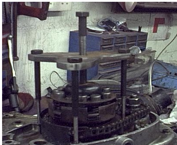
Clutch compressing tool using chain case bolts
