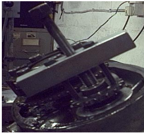
Sprocket puller on modified primary sprocket
